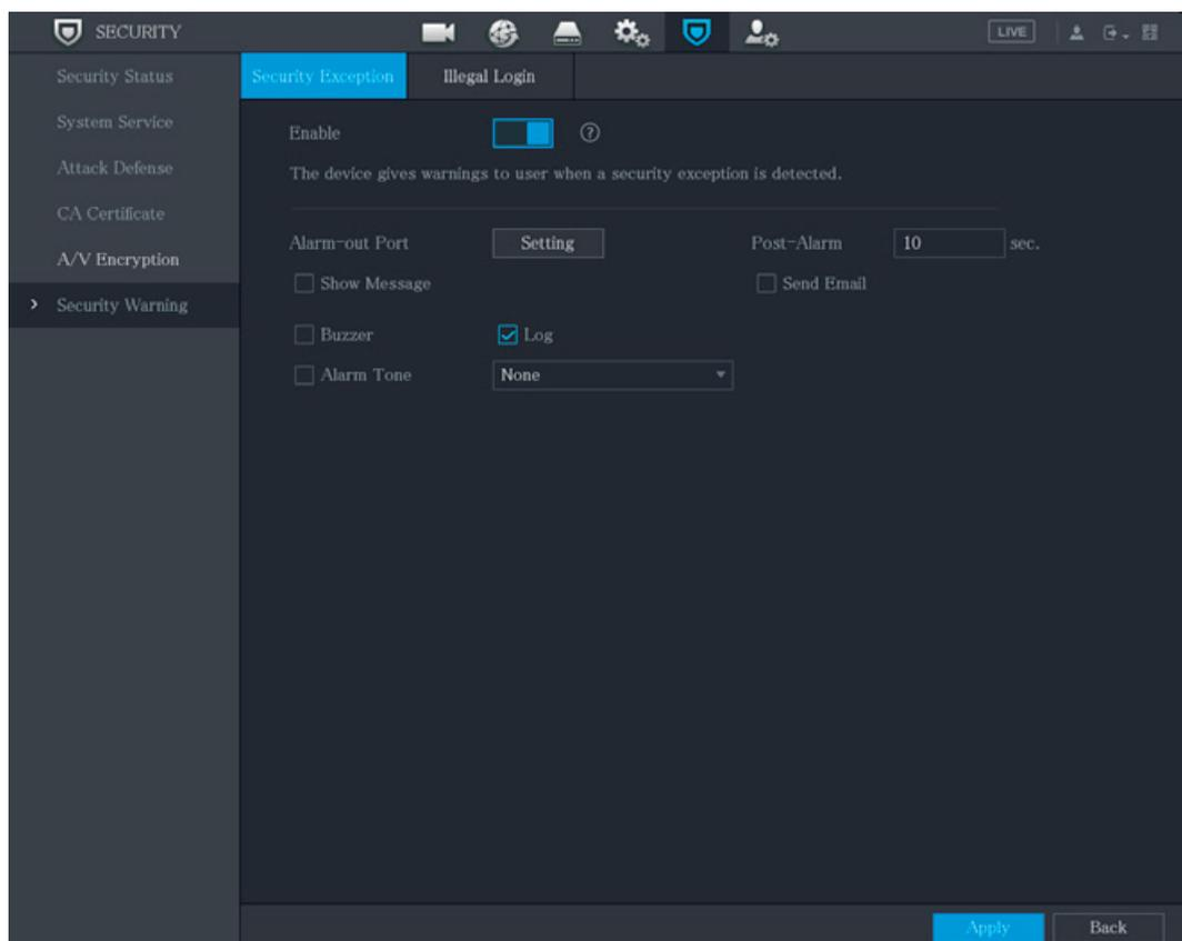
**Step 2** Select **Enable** and configure parameters.
