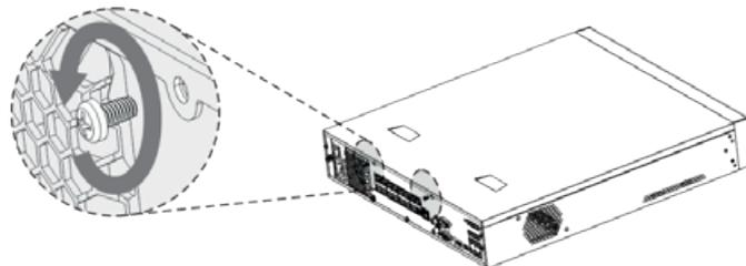
Step 2 Remove the cover along the direction shown in the following arrow.
