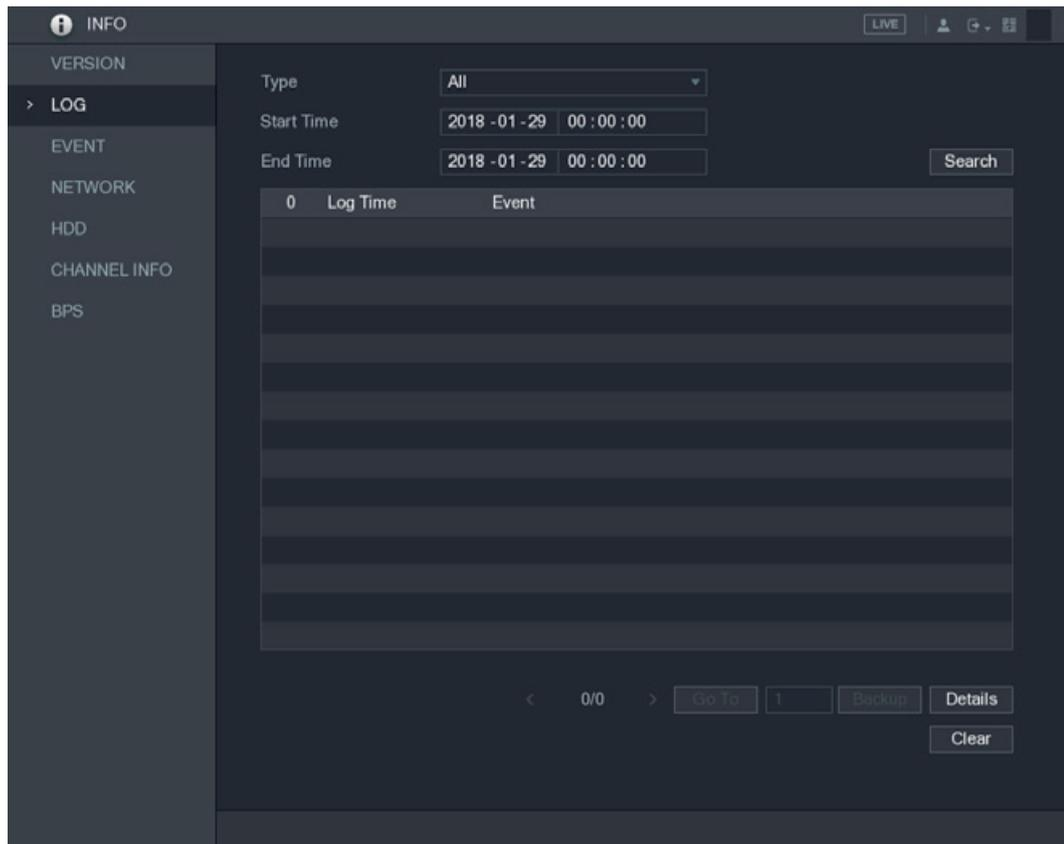
**Step 2** In the **Type** list, select the log type that you want to view (**System, Config, Storage, Record, Account, Clear, Playback, and Connection**) or select **All** to view all logs.
