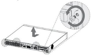
Step 2 Put two screws on the HDD and twist one turn. Figure 2-2 Put screws
