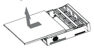
Step 3 Remove the screws from the drive bracket to take it off.
