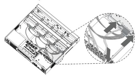
Step 8 Put back the cover and fasten the screws on the rear panel to complete the installation. Figure 2-23 Put back cover
