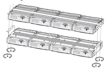
Step 7 Put the drive brackets back and fix them in the DVR. Figure 2-13 Put back drive bracket
