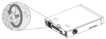
$\underline{\text{Step 2}}\ \ \text{Remove the cover along the direction shown in the following arrow.}$
